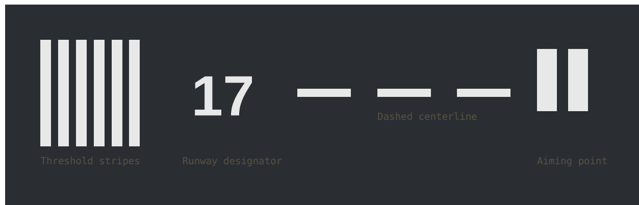
Fig 8.2 White runway markings: threshold bars, the runway designator, dashed centerline, and the fixed aiming-point blocks where you target your touchdown attitude. Taxiway markings are yellow.
